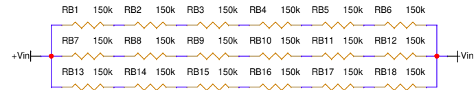
Safety Bleeder Resistors for Cap Bank
